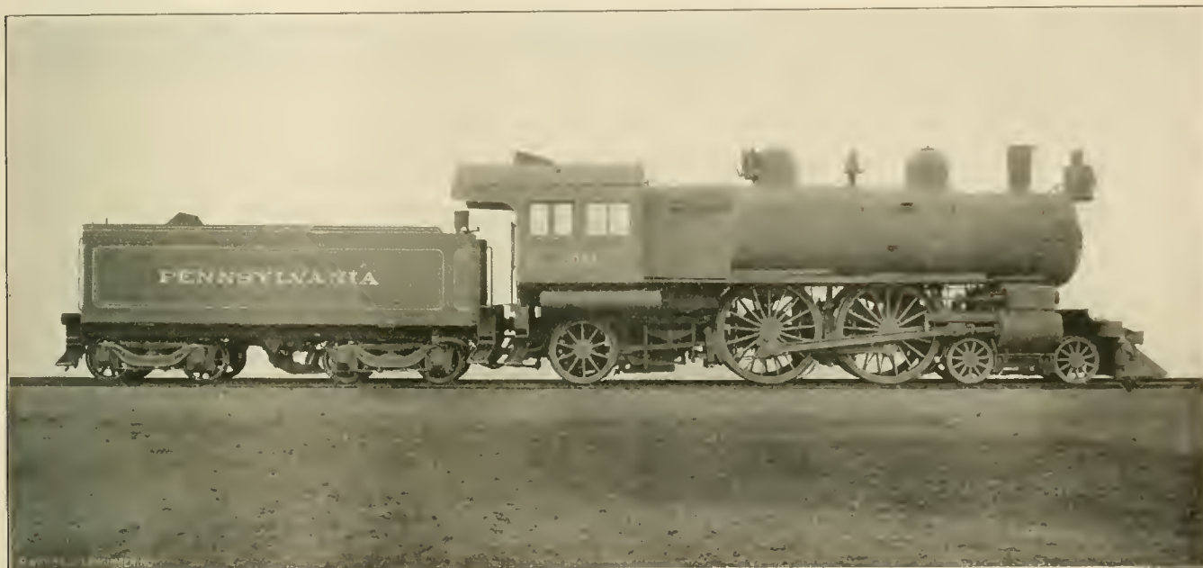
ATLANTIC TYPE ENGINE FOR THE PENNSYLVANIA, BUILT AT THE ALTOONA SHOPS.
